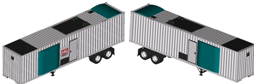
Figure 7: Ffowcs Williams–Hawkings (FW-H) sampling surfaces (green)
