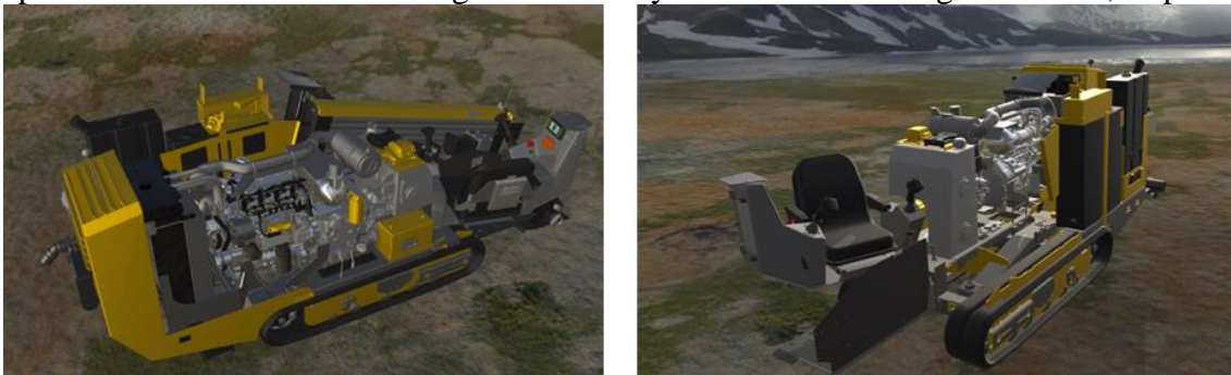
Figure 2: Directional drill, showing interior, engine, cooling package, exhaust and other underhood components
